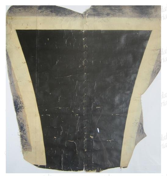
Section of clear doped fabric from the upper wing of a WW1 German aircraft.
