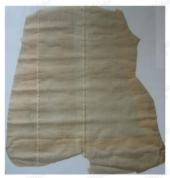
The condition of the fabric is excellent with very little flaking to the paint and the fabric is still relatively supple. The cross size would fit a single seater of the period, such as an Albatros DI/II or a smallish 2 seater such as an LVG or Albatros but there are numerous types it could be.
